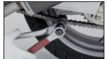
4a. Use a 27mm closed in wrench to hold firm the body of your chain tool while using a closed end 19mm wrench on the tool's hexagon bolt head to tighten. It will be easier to tighten the bolt if you position your wrenches 30° apart.
