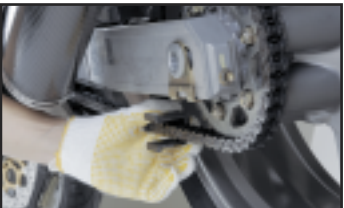
1a. Before cutting, loosen chain using your rear wheel adjusters. Position your KM500R or KM501E over your chain on the bottom side of your swingarm; cut the pin on the right side of the link you choose. If your chain has a master link, cut the chain at the master link.
