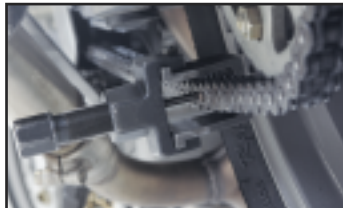
3a. To align the tool's Cutting pin with the chosen pin head, turn the tool's large bolt head clockwise "by hand" until the Cutting pin comes in contact with the pin head. At this point, make sure that the cutting pin is lined up with the center of the pin you wish to push out.
