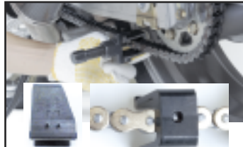
2a. Set the Cutting pin location on your chain tool's U-shaped holder to the point A position.
